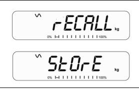
Press the [→Lim] key. If you are already in the check weighing mode the display will ask if you wish to store the current limits by showing "StOrE" or recall another set of limits by showing "FECALL". The [→Lim] key can be used to toggle between "StOrE" and "rECALL".
