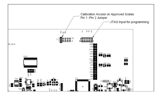
Apply power to the indicator. If the jumper has been used the display will ask for a code number, **"Pn"** on the Weight Display immediately. Or press the [Tare] key during the time the calibration counters are being displayed.
